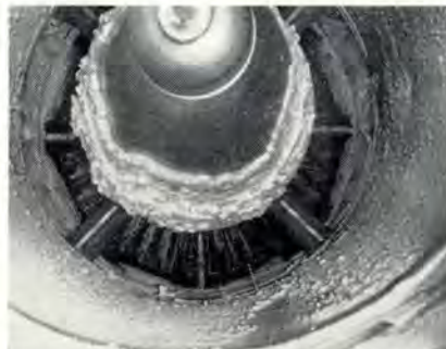
These pictures arrived too late for the B-47 article IN . . . AROUND . . . OVER . . . and THRU in the Feb. AEROSPACE SAFETY. Here they are—pictorial proof—B-47 engine icing tests.
