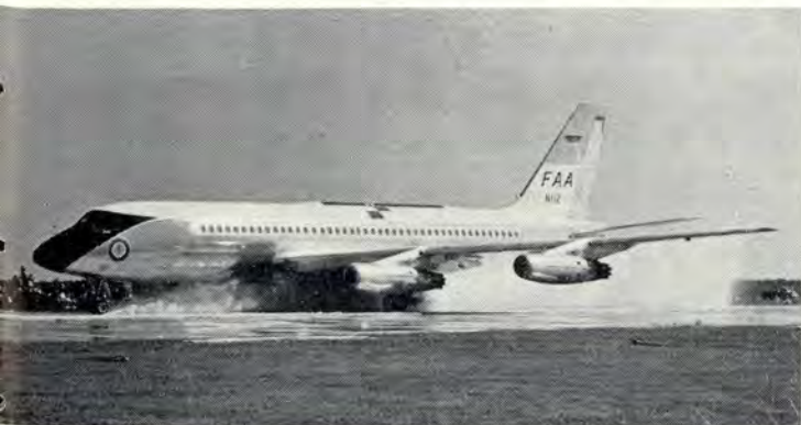
(3) Intermediate speed (135K) hydroplaning. No bow waves, small narrow spray pattern, little slush impingement, no direct tire-to-runway contact. (4) High speed (155K) hydroplaning. Note decrease in slush pattern from No. 1 with six leading wheels in intermittent runway contact.
