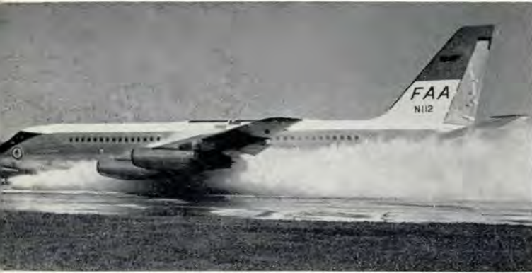
(1) Subplaning speed (80K). Heavy bow wave from main wheels throws slush in wheel wells and around inboard flaps. Heavy slush on fuselage, wing roots, flaps and tail. (2) Hydroplaning starts (120K). Smaller bow wave and spray pattern, less slush impingement. Nosewheels hydroplaning.
