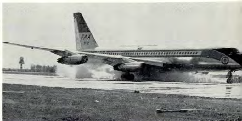
(3) Intermediate speed (135K) hydroplaning. No bow waves, small narrow spray pattern, little slush impingement, no direct tire-to-runway contact. (4) High speed (155K) hydroplaning. Note decrease in slush pattern from No. 1 with six leading wheels in intermittent runway contact.
