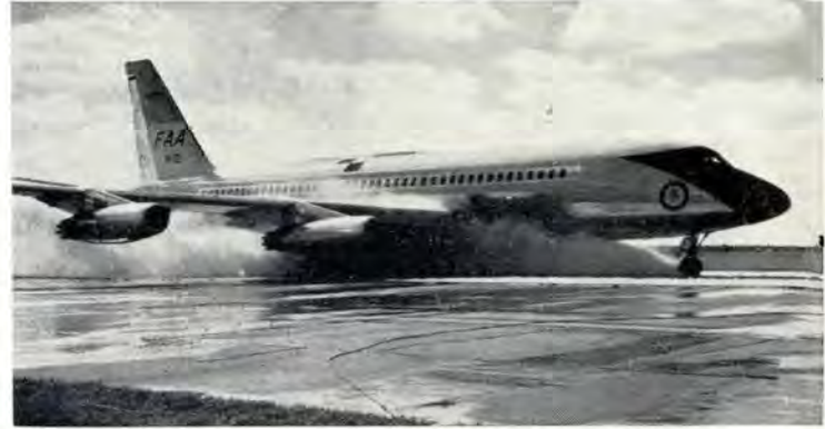
(1) Subplaning speed (80K). Heavy bow wave from main wheels throws slush in wheel wells and around inboard flaps. Heavy slush on fuselage, wing roots, flaps and tail. (2) Hydroplaning starts (120K). Smaller bow wave and spray pattern, less slush impingement. Nosewheels hydroplaning.
